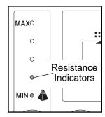
level 1 is selected; when the lowest indicator is brightly lit, resistance level 2 is selected; when the second indicator is dimly lit, resistance level 3 is selected; when the second indicator is brightly lit, resistance level 4 is selected; and so forth. When the highest indicator is brightly lit, resistance level 10, the most difficult level, is selected.
